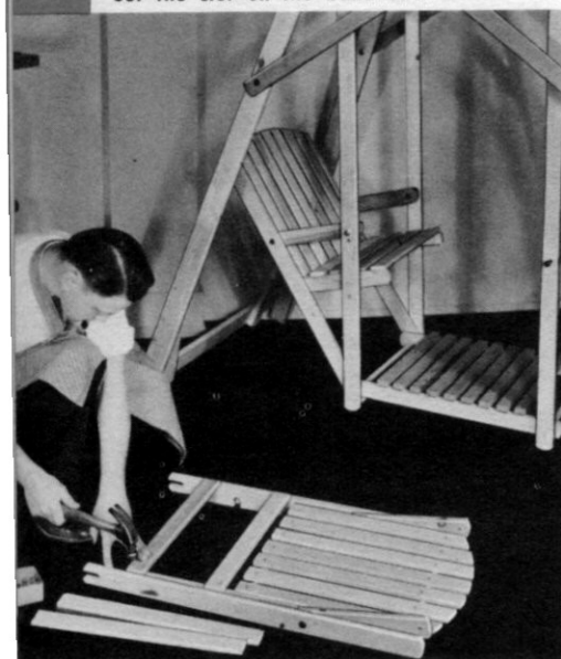
The above photo shows the seat being assembled with lath nails.
