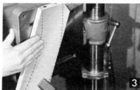
Mark off the dowel hole positions on the angle cuts of each arch section and bore 5/16-inch holes. Stock is held in position on the drill press with the table tilted to 90 degrees. Pieces are clamped to table with handscrews.
