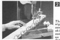
The scrolled trim design is cut on the band saw using a 1/4-inch skiptooth blade. These same cuts can be made on the scroll saw, if desired.
