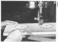
Holes are cut on the scrollsaw with the No. 92 jeweler's blade running the machine at 1725 rpm. The holes may also be bored on the drill press with an adjustable hole cutter.
