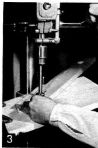
1-1/4" holes are bored on the drill press using a multi-spur bit. The jig board (Fig. 4) is mounted to the drill press table with C-clamps and the drill press table tilted 15 degrees.
