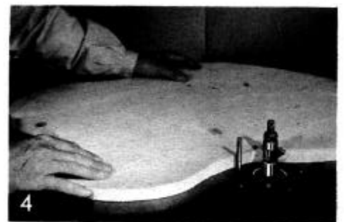
The table top edge is free hand shaped on the spindle shaper with the No. D-103 three-lip cutter. The start of the moulding is made against the taper starting pin.
